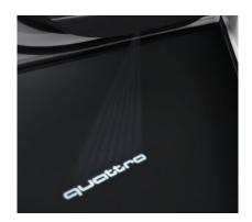
The entry LED projects the quattro lettering onto the ground when the front doors are opened.
