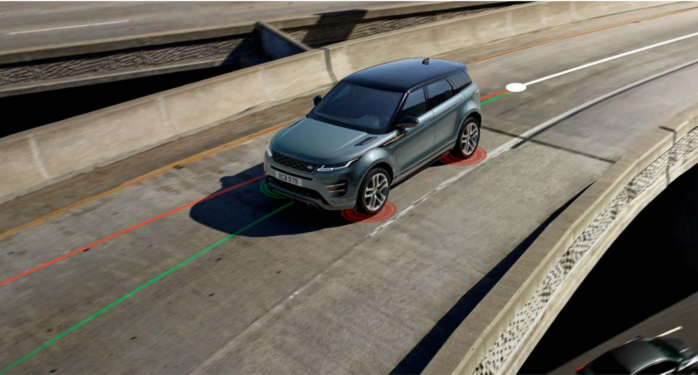
— UNDERSTEER DETECTED — FULL TORQUE TO OUTER WHEELS ● UNDERSTEER DETECTED ● FULL TORQUE TO OUTER WHEELS
