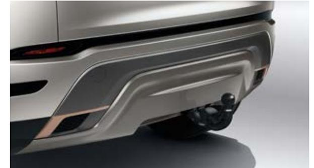
Electrically Deployable Tow Bar
