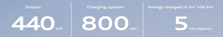
Up to 270 kW at 800-volt charging stations – as standard. It takes approx. 5 minutes to charge enough power for the next 100 km. Around 22.5 minutes will take the battery charge from 5 % back up to approx. 80 %.
