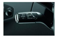
Retrofit solution for the cruise control system maintains any speed as of approximately 30 km/h.
