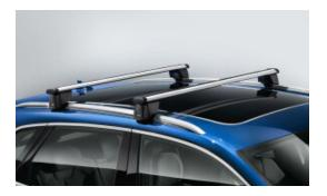
Roof carrier of powder-coated, aerodynamically formed aluminum profile with plastic mounting elements.
